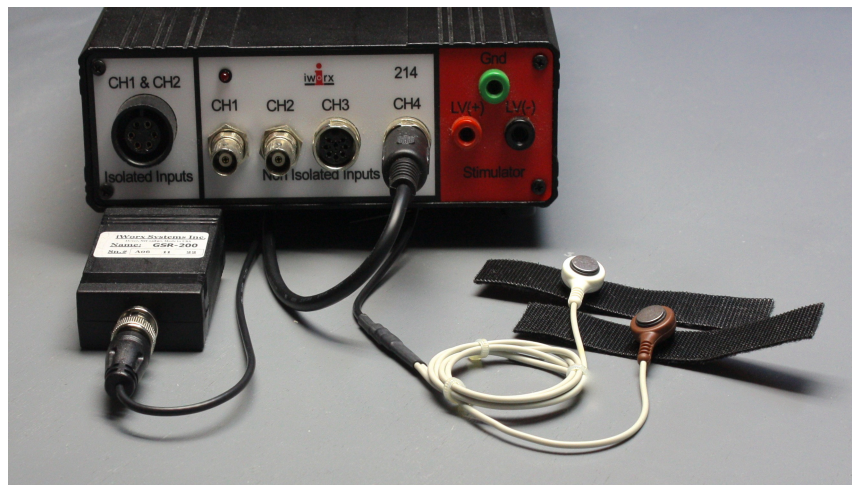
Figure HP-3-S2: The GSR-200 connected to an IWX214.
